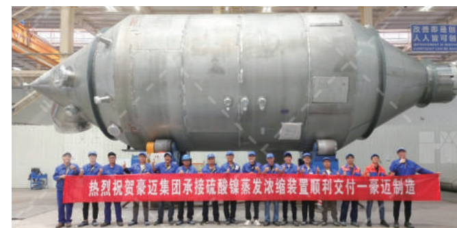
哈氏合金、超级双相不锈钢、双相不锈钢等特材加工的蒸发浓缩装置 Evaporation and concentration unit with Hastelloy, super duplex SS, duplex SS
