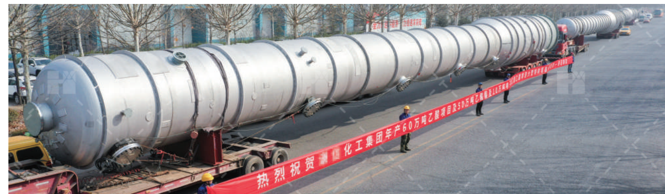
负压重组分塔 (DN3800×81470) Vacuum Heavy Fractionation Tower
