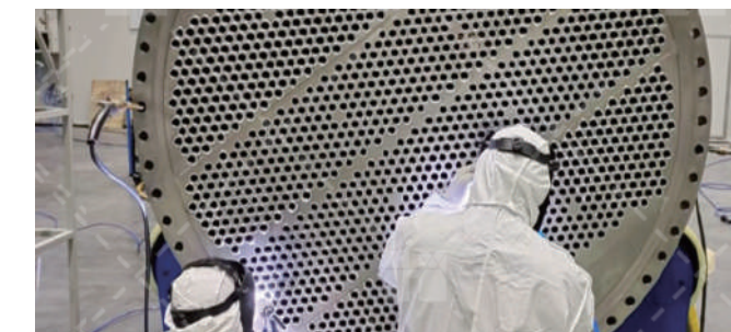
钛合金再生气热交换器 regas heat exchanger with Titanium alloy
