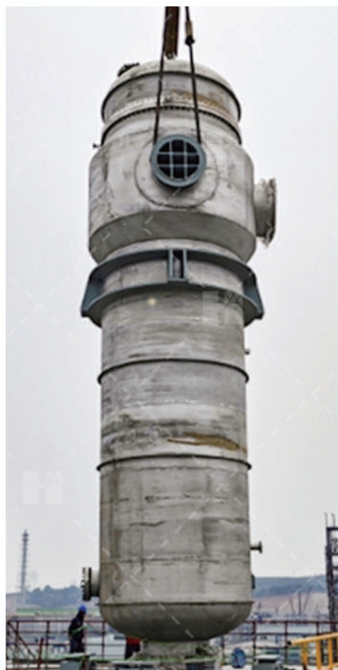
多效降膜再沸器 DN3200×10000mm Multi-effect falling film reboiler
