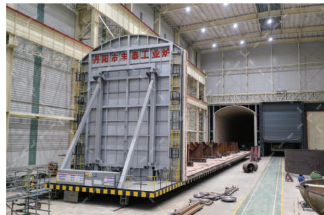
热处理炉 (尺寸 51×11.5×13m; 允许最大工件50*10.5*12米; 热处理台车牵引力最大1200t) Heat treatment furnace (dimension 51000mm×11500mm×1300mm, Maximum Workpiece Dimensions 50*10.5*12m, Heat Treatment Car Pulling Force Max.1200t.)
