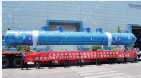
低压加热器 Low-Pressure Heater
