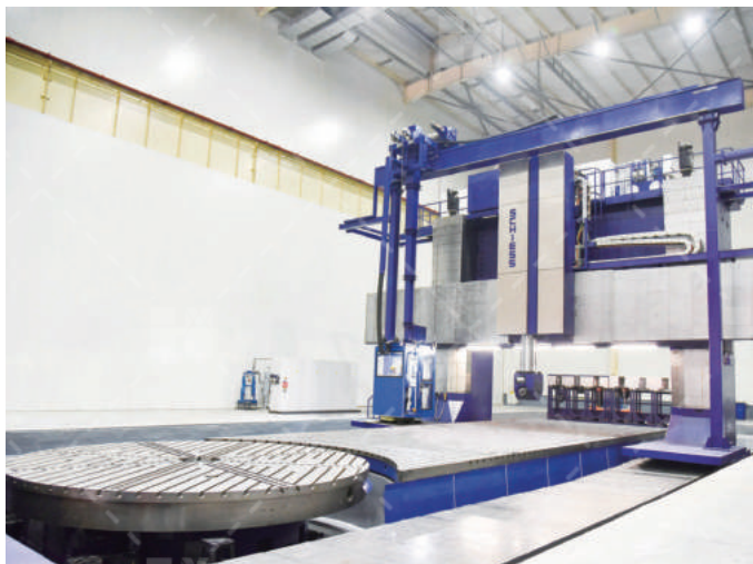
希斯龙门 (加工范围:21000×8000×5000mm) SCHIESS Gantry Machine (Working range: 21000×8000×5000mm)
