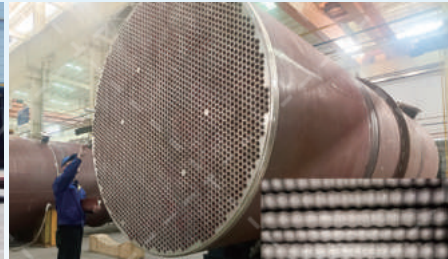
波纹管热交换器 DN2700×14380mm Corrugated Tube Heat Exchanger
