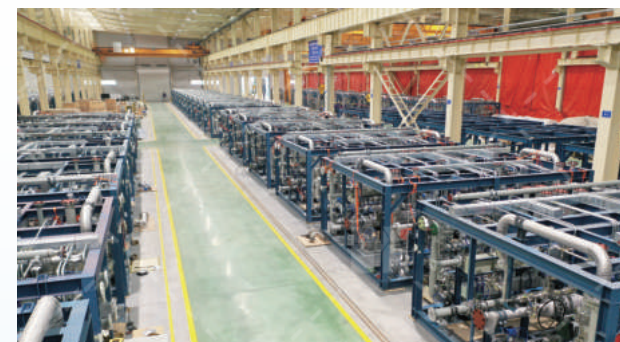
多晶硅还原炉撬块 CVD Reactor Skid
