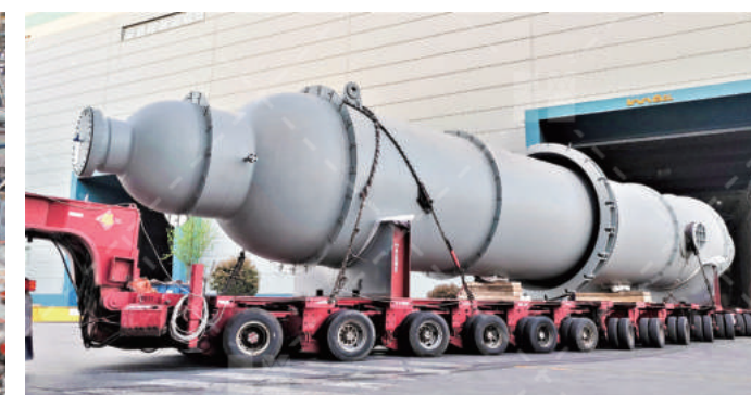
乙酸甲酯-粗醇换热器 (DN2800×14800) Methyl Acetate-Crude Glycol Heat Exchanger
