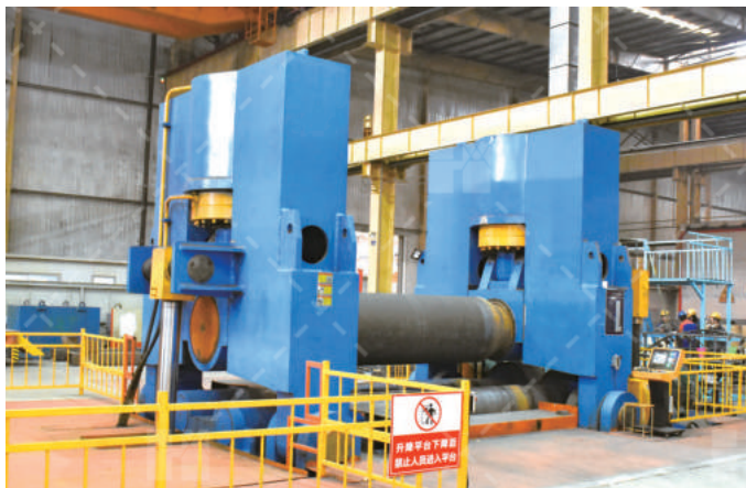
200mm卷板机 200mm plate rolling machine
