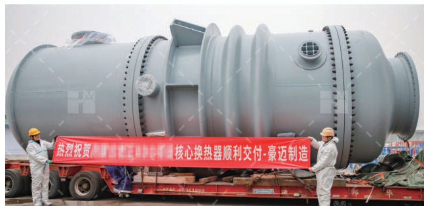
循环塔列管再沸器 DN3500×11000mm Circulating tower reboiler
