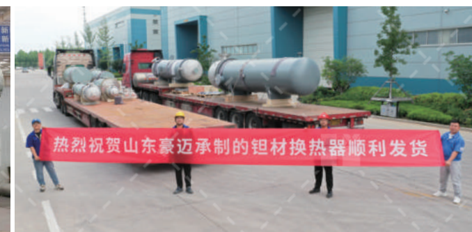
钽材酸浓缩热交换器 Tantalum acid concentration heat exchanger
