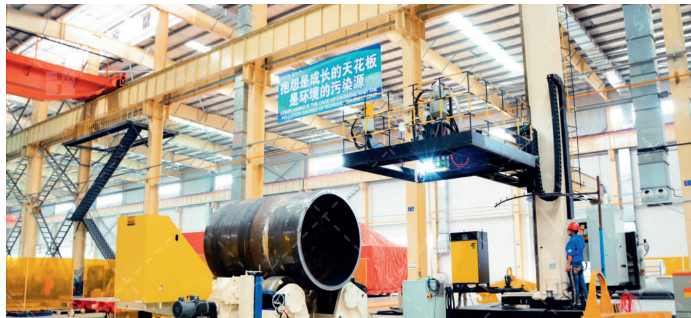
大壁厚、窄间隙埋弧焊机 (最大焊接厚度300mm) Large Wall Thickness and Narrow Gap SAW Machine (Max. welding thickness is 300mm)
