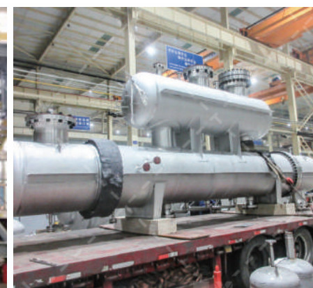
组合式热交换器 DN1200×4500mm Combined heat exchanger
