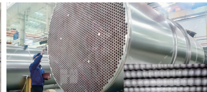
镍基合金氧汽提塔回流热交换器 Oxygen tower reflux heat exchanger with nickel-based alloy
