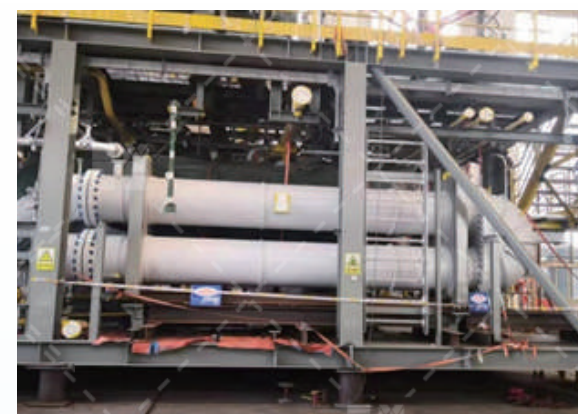
发卡式热交换器 DN700×6392mm Hairpin heat exchanger
